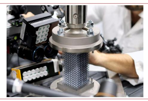
DIC is an optical measurement technique that measures displacement and strain fields by following a pattern in a series of images
